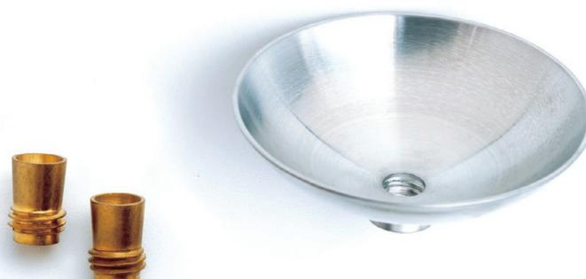
K30500 Float Test Apparatus
