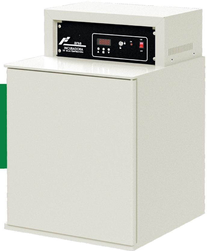
*The low temperature incubator is ideal for any laboratory where wastewater BOD testing, fermentation studies, enzyme assays, and drug stability testing, among other applications, are common. Digital control and internal chamber with forced air circulation.*
