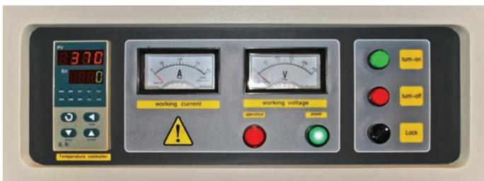
**DOBLE DISPLAY** - Control de temperatura digital universal P.I.D., autotuning.
